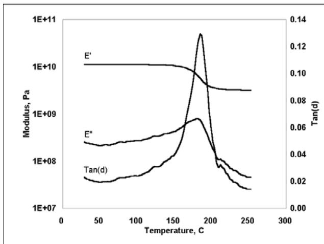
**Figure 3. Style 181 Fiberglass with Tactix 123/OPPI (3 phr)**
