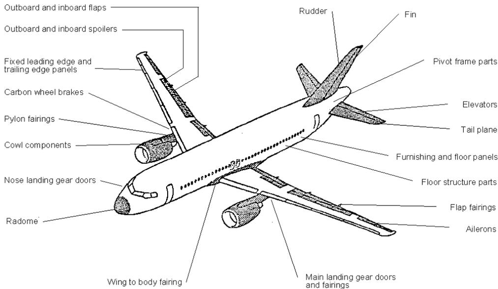
Air Canada plans to perform a number of repair type-trials on various composite components. These type-trials will evaluate the feasibility and economics of EB processing for repair. For the first type-trial, a fairing of a A320 aircraft will be repair tested. This particular component, constructed of fiberglass and a thermal-cured epoxy resin, is located at the lower rear of the aircraft
